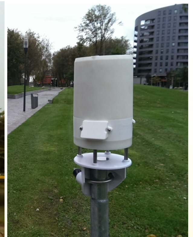
Mock-up of TAHMO MEM Station
